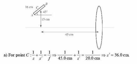
$y' = -\frac{s'}{s}y = -\frac{36.0}{45.0}(15.0 \text{ cm}) = -12.0 \text{ cm}$ , so the image of point C is 36.0 cm to
